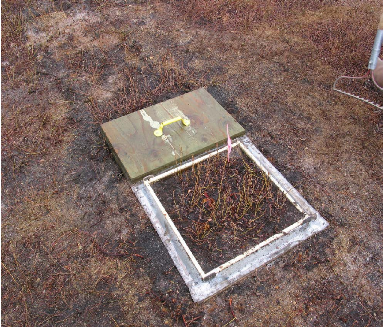
Figure 1. A weighing lysimeter containing newly transplanted blueberry sod.
