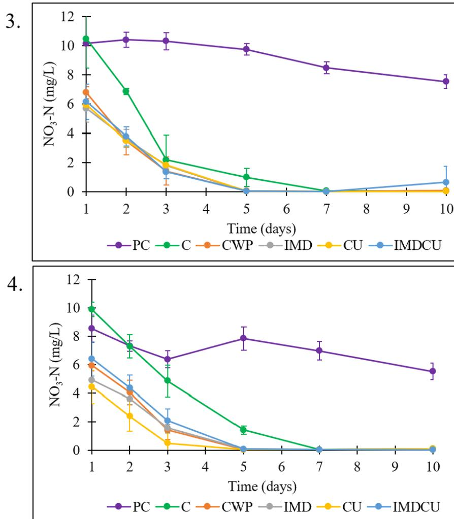
Figure 3. NO<sub>3</sub>-N loss in mesocosm wetlands over the 10-day sampling period during (a) experiment 1 at 0 ng/L, (b) experiment 2 at 50 ng/L, (c) experiment 3 at 500 ng/L, and (d) experiment 4 at 1,000 ng/L.
