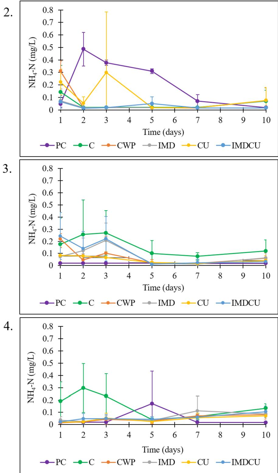
Figure 4.  $\text{NH}_4\text{-N}$  loss in mesocosm wetlands over the 10-day sampling period during (a) experiment 1 at 0 ng/L, (b) experiment 2 at 50 ng/L, (c) experiment 3 at 500 ng/L, and (d) experiment 4 at 1,000 ng/L.
