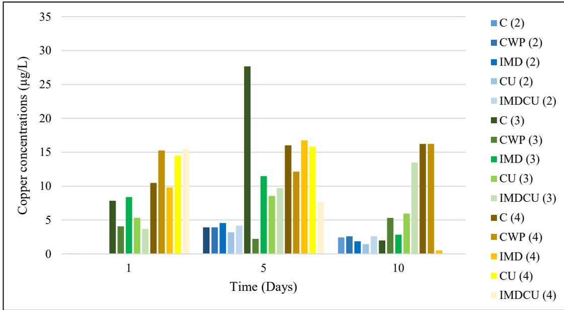
Figure E.1. Undigested copper concentrations in experiment 2 at 50 ng/L (blue), experiment 3 at 500 ng/L (green), and experiment 4 at 1,000 ng/L (yellow).
