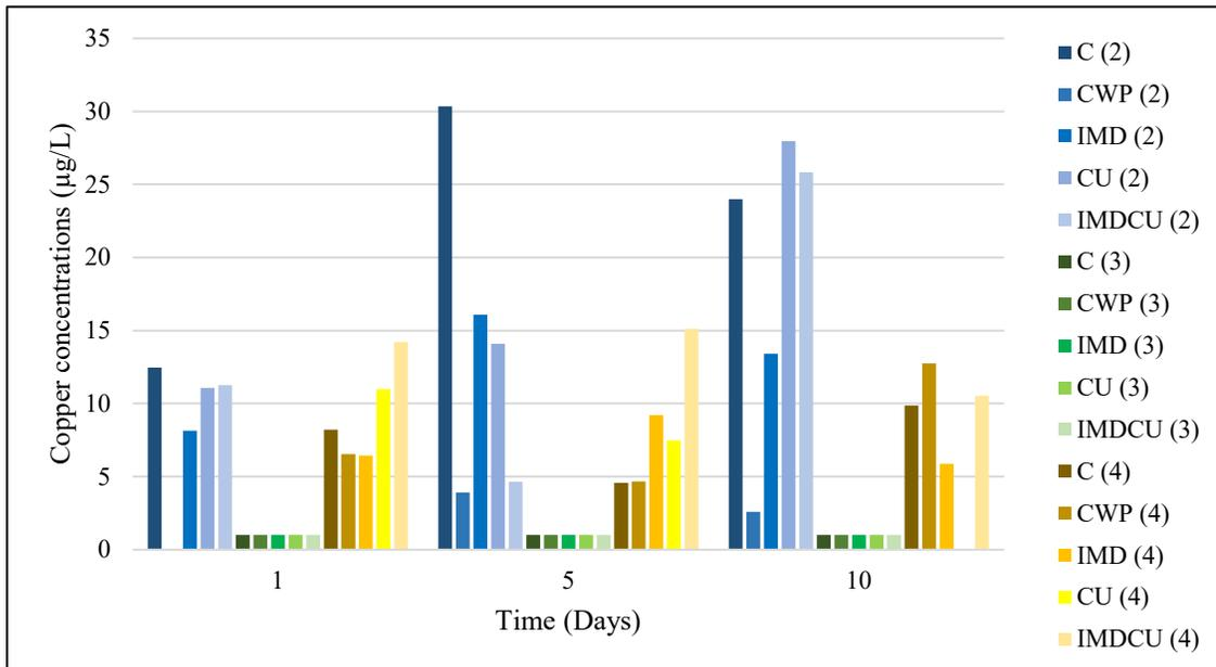
Figure E.2. Digested, filtered copper concentrations in experiment 2 at 50 ng/L (blue), experiment 3 at 500 ng/L (green), and experiment 4 at 1,000 ng/L (yellow). Samples C1-IMD1 of experiment 3 were not analyzed for Cu on days 1,5, and 10.
