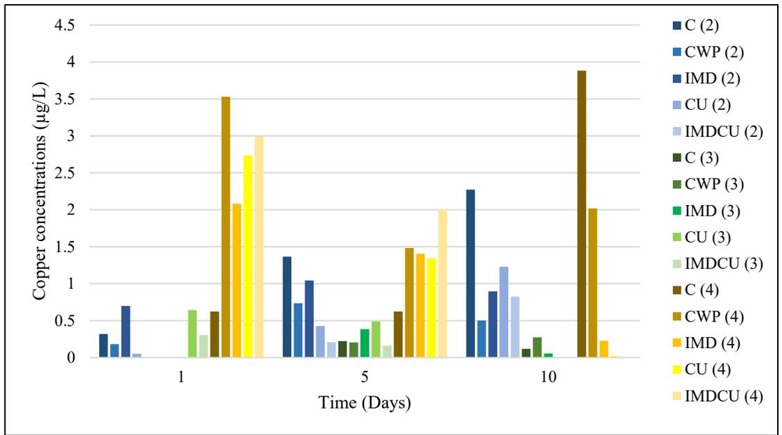
Figure E.3. Digested, unfiltered copper concentrations in experiment 2 at 50 ng/L (blue), experiment 3 at 500 ng/L (green), and experiment 4 at 1,000 ng/L (yellow).
