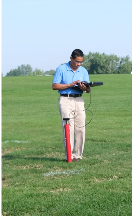
Figure A 3: Clegg Impact Hammer in use at turfgrass test plots
