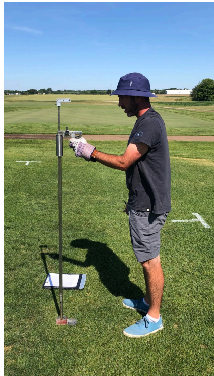
Figure A 4: Longchamp Penetrometer in use at turfgrass test plots
