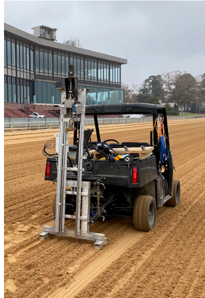
Figure A 1: Orono Biomechanical Surface Tester on a dirt racetrack
