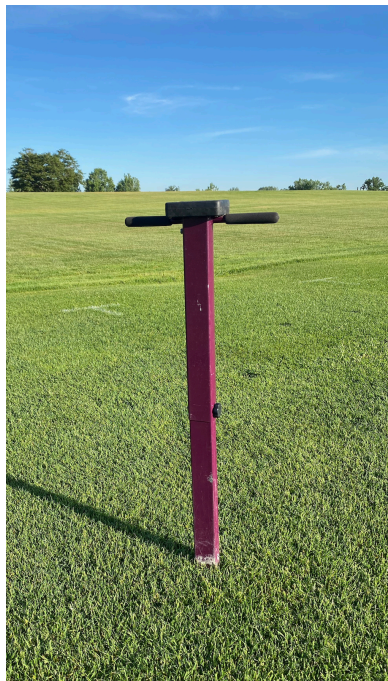
Figure A 2: TDR 350 moisture probe in use at turfgrass test plots
