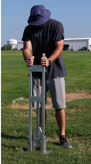
Figure A 5: Turf Shear Tester in use at turfgrass test plots
