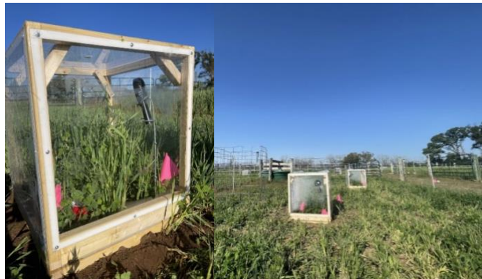
Figure 1. Chambers used for 13 CO 2 cover crops labeling in North Florida.
