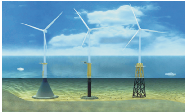
(a) Gravity structure (b) Monopile (c) Jacket
