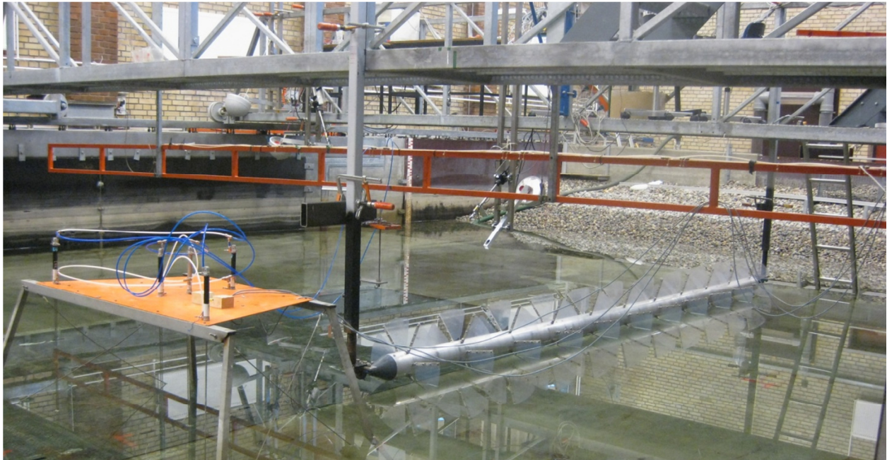
Figure 1. Laboratory setup for Rolling Cylinder long model in scale 1:25.
