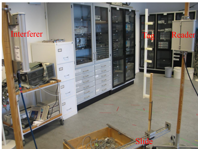
(a) The reader and interferer antennas with the tag in between.
