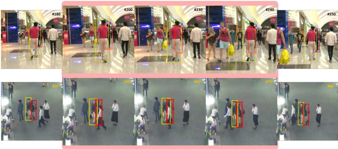
Figure 27: Tracking occluded object (red bounding box) by its relations with neighbors. The position of the object in the shaded region is recovered from its relation embedding.
