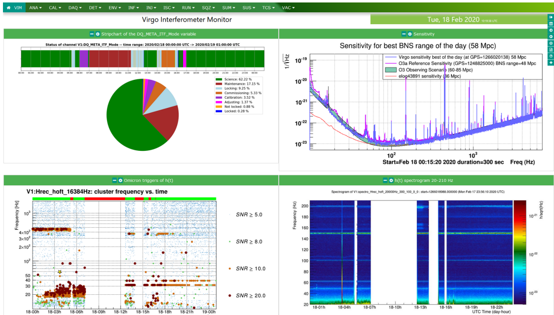
Figure 4. Screenshot of a VIM web page displaying information about the Virgo detector on Tuesday February 18 th , 2020. Top left plot, stripchart of the detector status: the weekly maintenance, preceded by a planned calibration and followed by a short commissioning period, interrupts the data taking that restarts in the evening. Top right plot: daily sensitivity compared with references. Bottom left plot: glitch monitoring provided by the Omicron analysis described in section 4.1. Bottom right plot: spectrogram of the GW strain h(t) in the 20-210 Hz frequency range.
