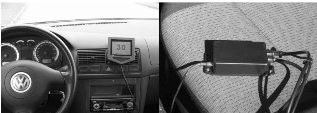
Figure 3.1. The display with a loudspeaker (left), and the OBU, which was normally mounted under the dashboard (right).
