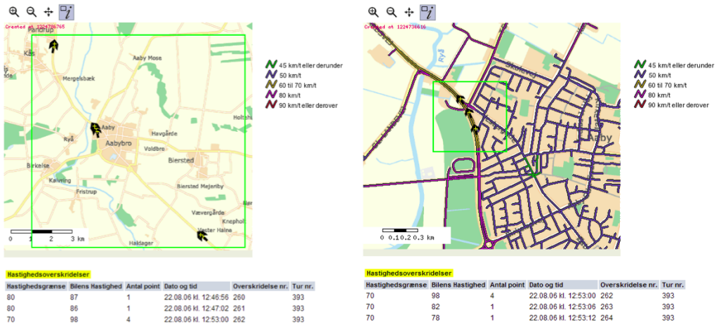
Figure 3.3. An example of feedback to a driver in case of penalty points with a small-scale overview (left) and a large-scale overview and visible speed limits (right).
