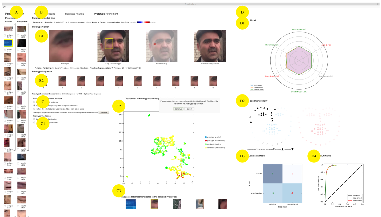
Figure 5. ProtoExplorer, a prototype based Visual Analytics system for analyzing deepfake videos, showing the model exploration and refinement screen . The list of prototypes (A) can be viewed in detail (B) and revised through deletion, replacement, or addition of prototypes (C), the impact of which can be observed in the performance panel (D).
