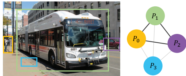
Figure 1. Problem Setting. From proposals, a graph is constructed and its edge weights are determined and assigned using prior knowledge. Redundant proposals (e.g. in blue) receive low edge weights due to their limited contextual relevance to other objects in the scene. As a result, less contextual feature information from neighboring nodes is aggregated to and from these proposal nodes, which eventually removes them from the final prediction.
