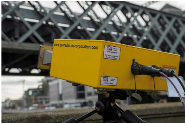
Figure 2. Interferometric radar set up at the Loopline Bridge.
