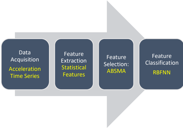
Figure 1. Summary of damage detection approach
