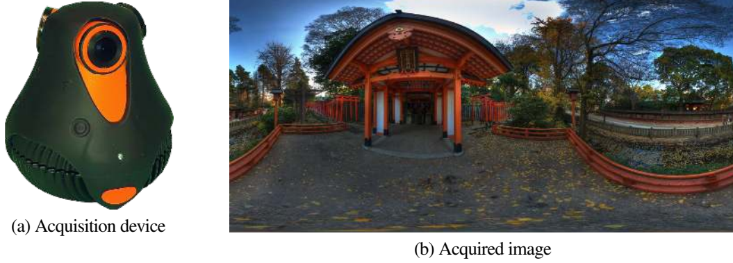
Figure 2.2: Acquisition device and obtained equirectangular panoramic image.
