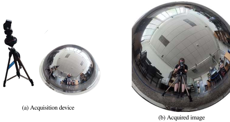
Figure 2.9: Acquisition device and obtained non-central catadioptric image with spherical mirror.
