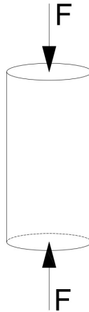
Figure 7: The principle for uniaxial compressive testing. The load is applied to the whole top and bottom end's surface
