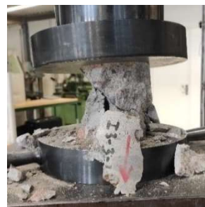
Figure 41: Core sample after compression test (2); load rate of 10kN/s
