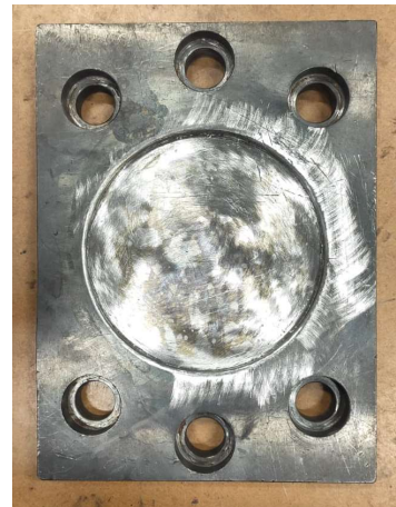
Figure 24: Loading plate, where the core sample is glued using X60-NP
