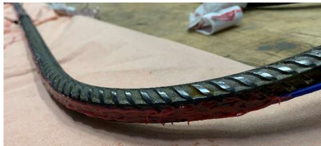
Figure 19: FOS installed and glued to a reinforcement steel bar
