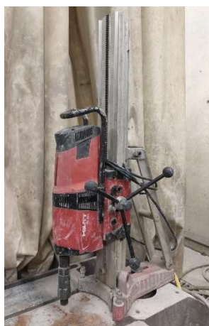
Figure 37: Diamond coring tool for wet drilling Hilti DD 200-CA Core Drill
