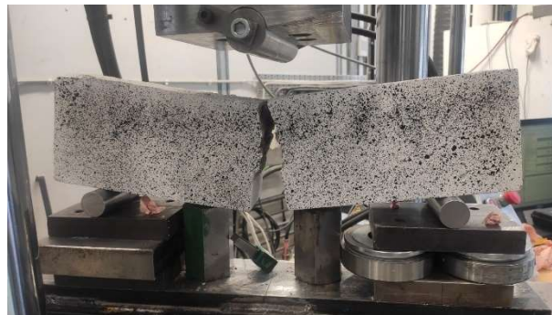
Figure 42: Cast concrete beam after 3PBT
