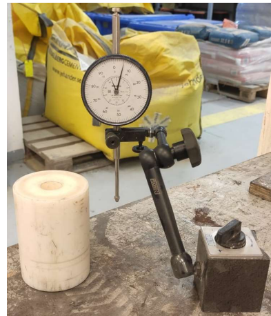
Figure 22: Dial gauge (right) and the 70mm diameter form (left) used for calibrating
