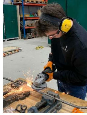
Figure 16: Bar polishing process in order to glue a strain gage
