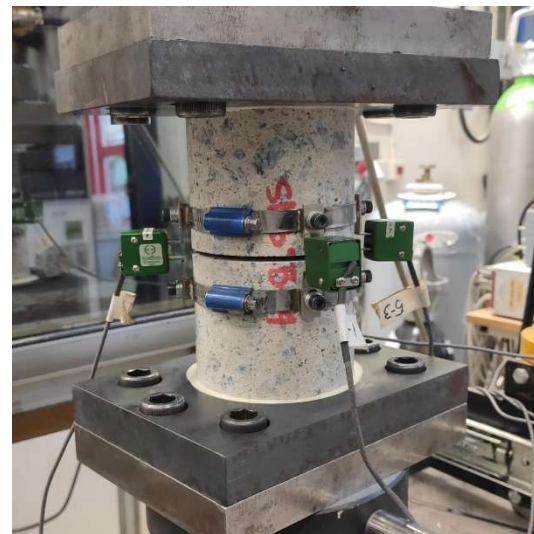
Figure 29: Tensile test layout for a concrete core (2)
