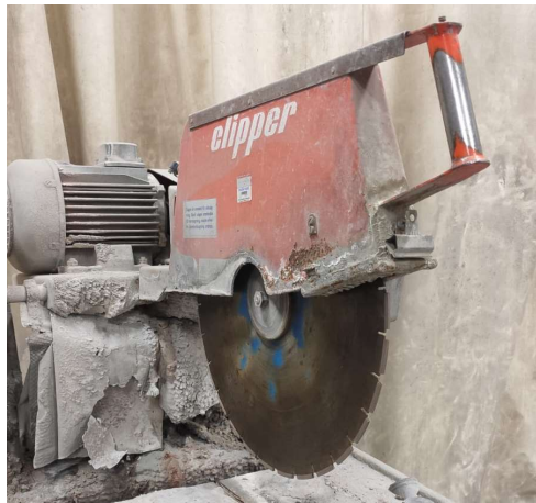
Figure 21: Saw used for cutting the ends of the core samples
