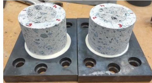
Figure 47: Core sample after tensile test is performed (2)
