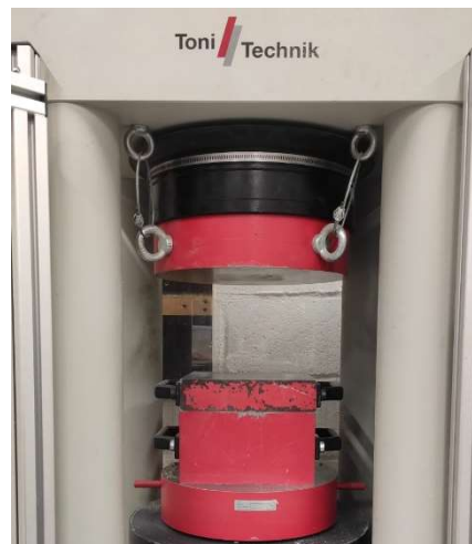
Figure 30: Hydraulic press used for Compressive tests
