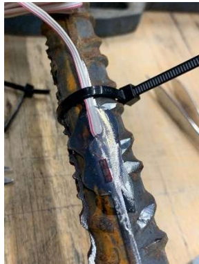
Figure 17: Strain gage glued to a reinforcement bar
