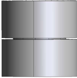
Figure 80: Example of notched concrete core developed with FEM
