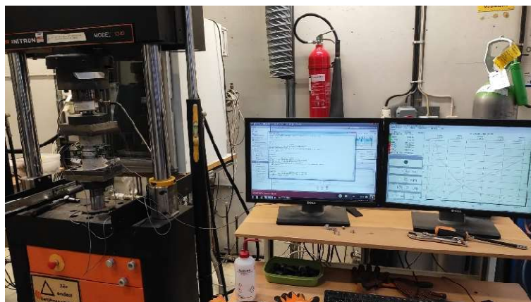
Figure 25: Direct tensile test being performed and monitored in real time
