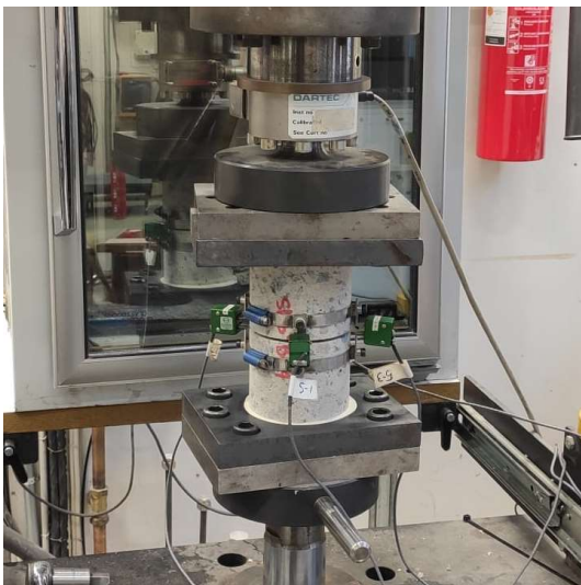
Figure 28: Tensile test layout for a concrete core (1)
