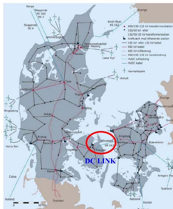
Figure 3.1 - East and West Danish electricity transmission grid in 2030 according to Energinet.dk's cable action plan [3]
