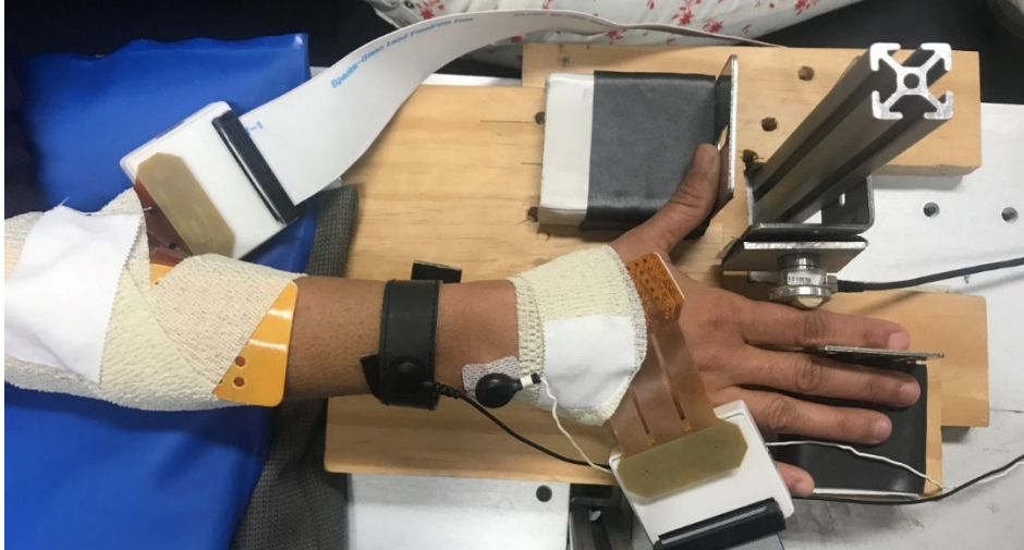
Fig 2.1: Experimental set-up for the index finger abduction task. The PIP joint is aligned with the wooden dowel to perform the abduction task. Movement of the thumb and other fingers is restricted due to the manipulandum.
