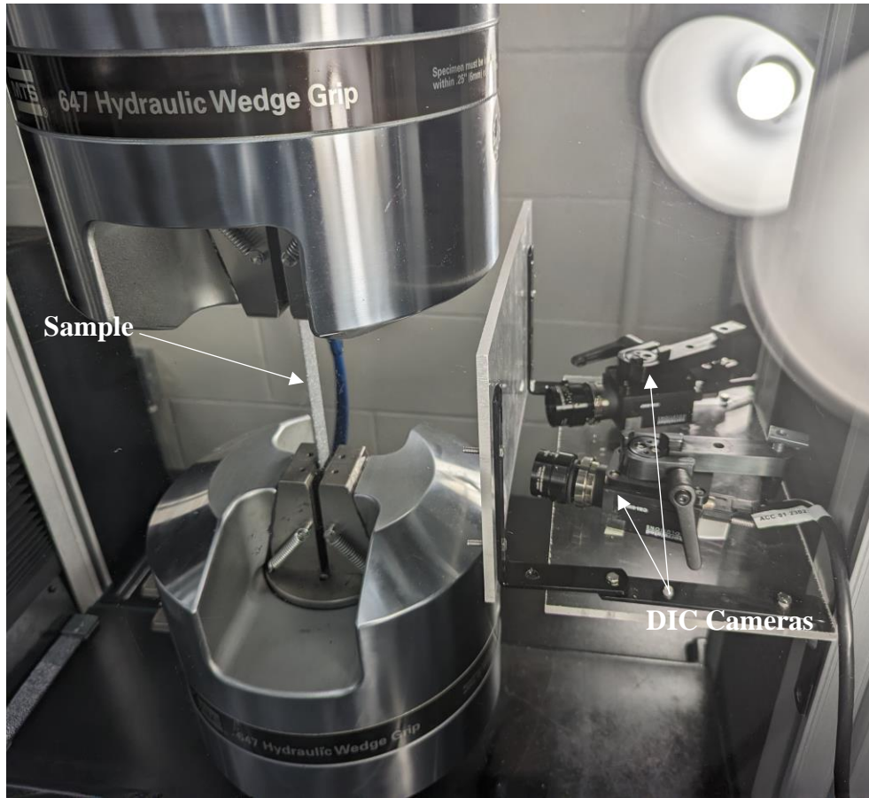
Figure 3.15 Sample fixture and DIC setup positioning
