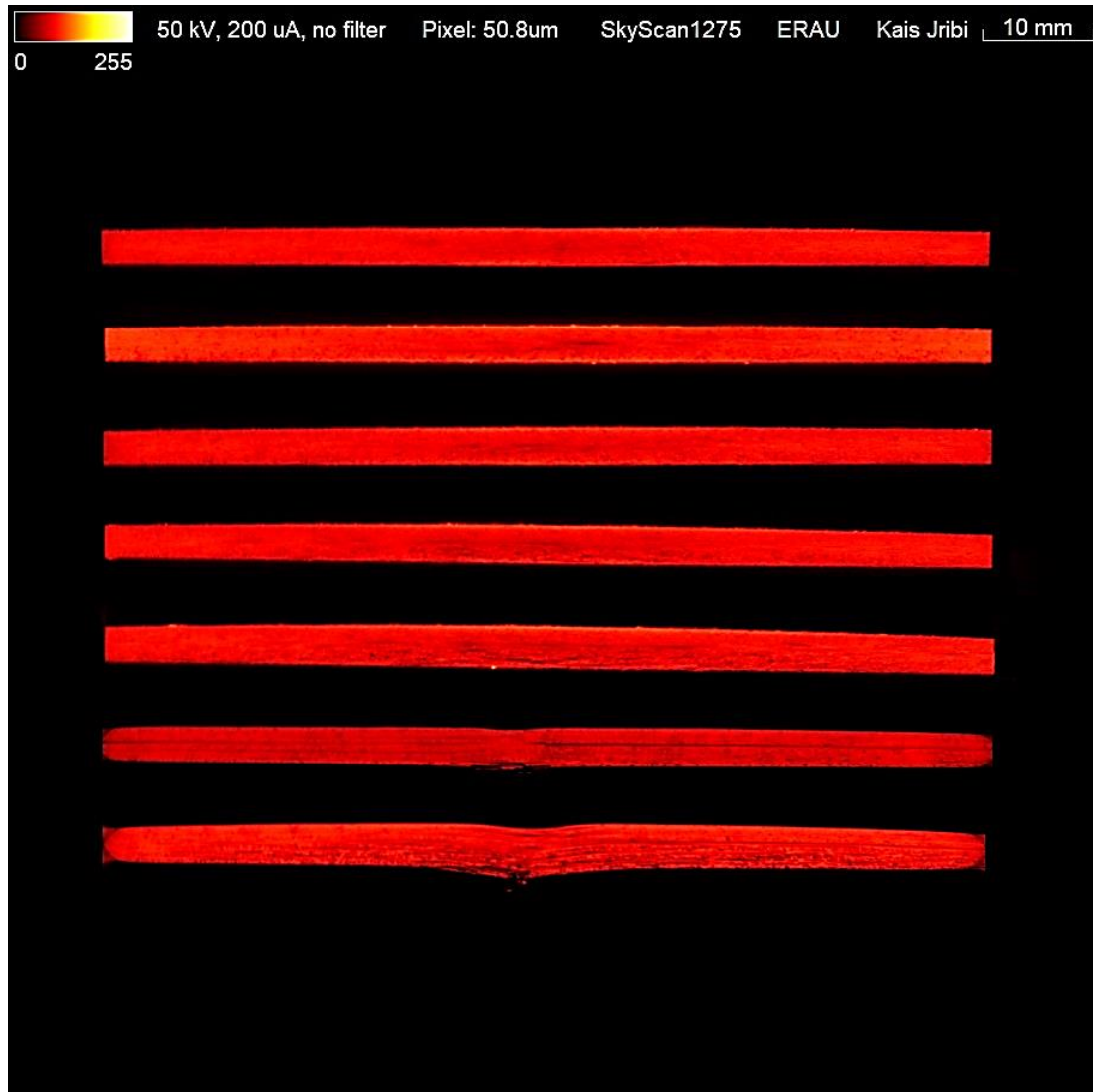
Figure 3.33 Damage profiles from LVI with different energy levels (from the top: 2.5J, 5J, 7.5J, 10J, 12.5J, 15J and 20J)
