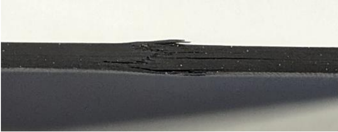
Figure 4.3 Structural failure in CFRP due to excessive compressive loads.
