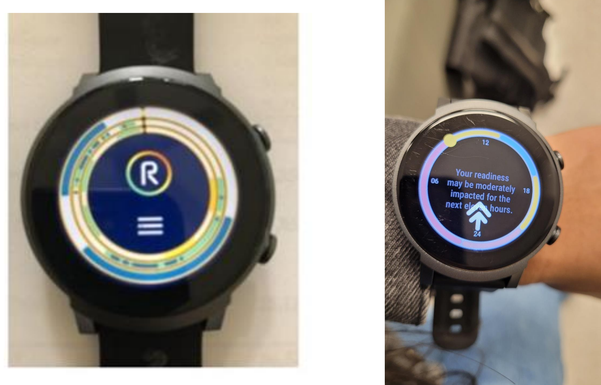
Figure 1. COTS smartwatch with app shows real time fatigue information at a glance based on sleep quality history
