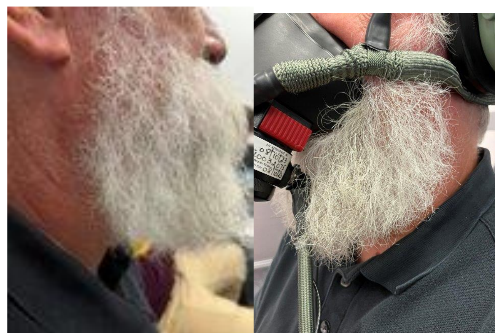
Figure 1. Example of >10mm beard fit of the Sweep-On 2000 crew oxygen mask system
