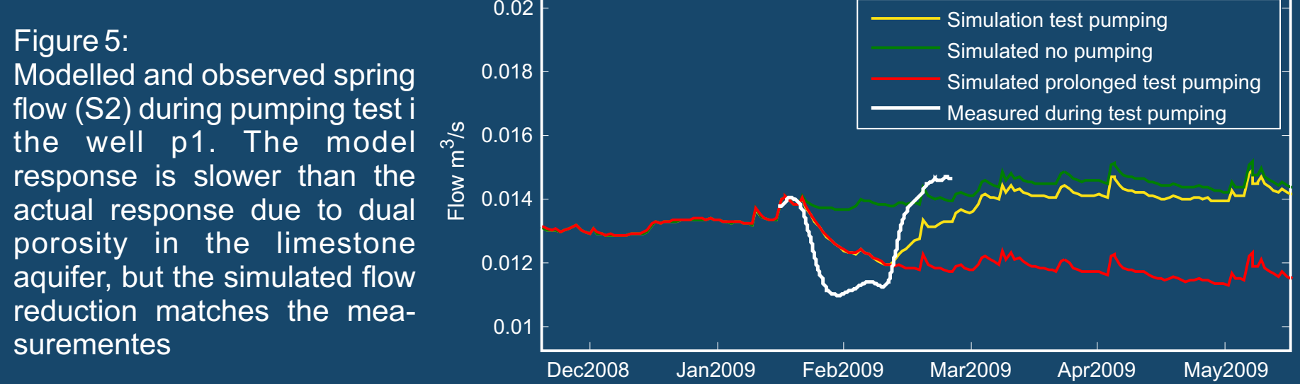
Figure 5: Modelled and observed spring flow (S2) during pumping test at the well p1. The model response is slower than the actual response due to dual porosity in the limestone aquifer, but the simulated flow reduction matches the measurements
