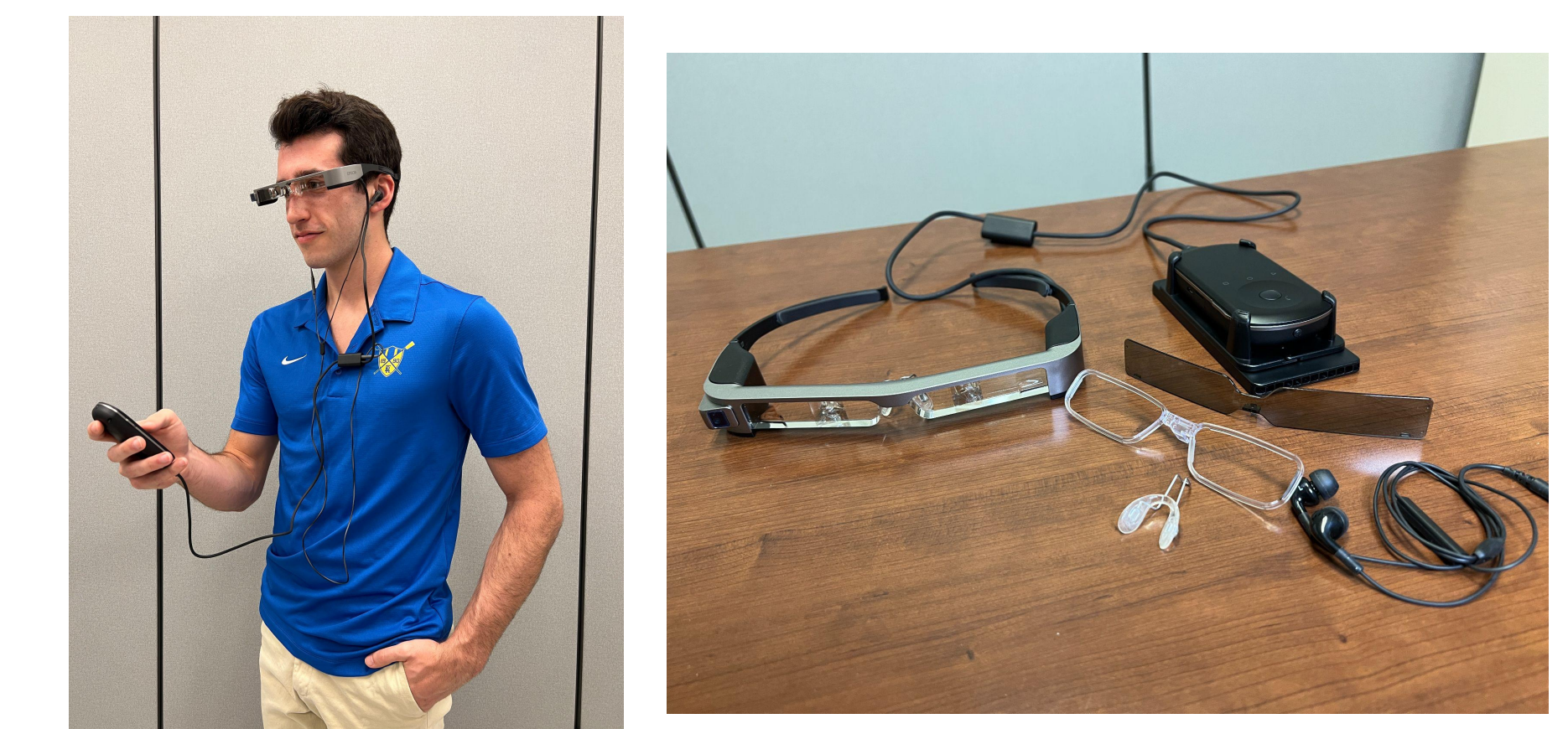
Figure 3. Epson Moverio BT-300 with Teather, Shade and Prescription Lense, Headphones, and Nose Inserts.
