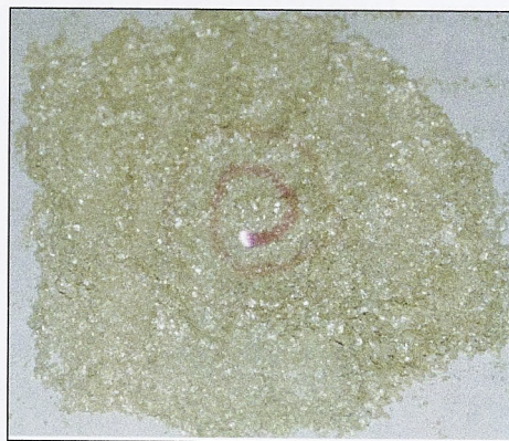
Figure 4. Molecule 4 selectively irradiated using a blue laser pointer (405 nm) to produce a spiral, illustrating the short lifetime of the red trans-keto form.
