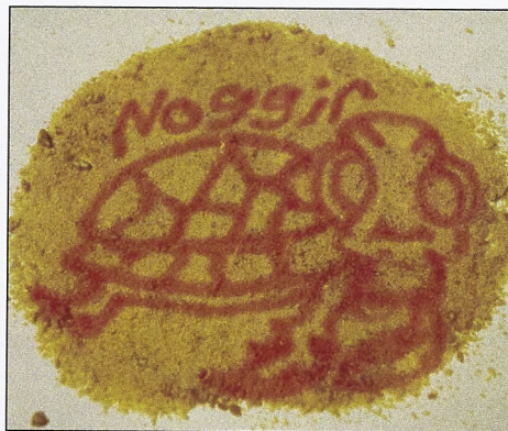
Figure 3. Molecule 1 selectively irradiated using a blue laser pointer (405 nm) to produce a complicated image.
