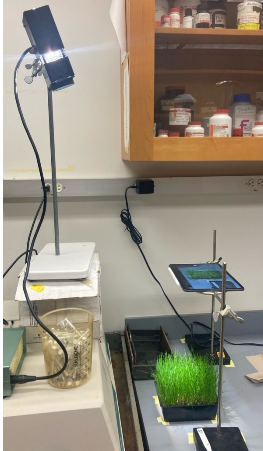
Figure 5. Digital photo set-up for turfgrass image analysis. Digital photos were taken with an iPad from the same position, lighting, and height each day to ensure consistency.
