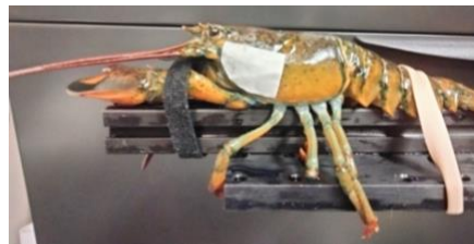
Fig. 5. American lobster strapped to a weight with reflective tape on the carapace for laser vibrometry.
