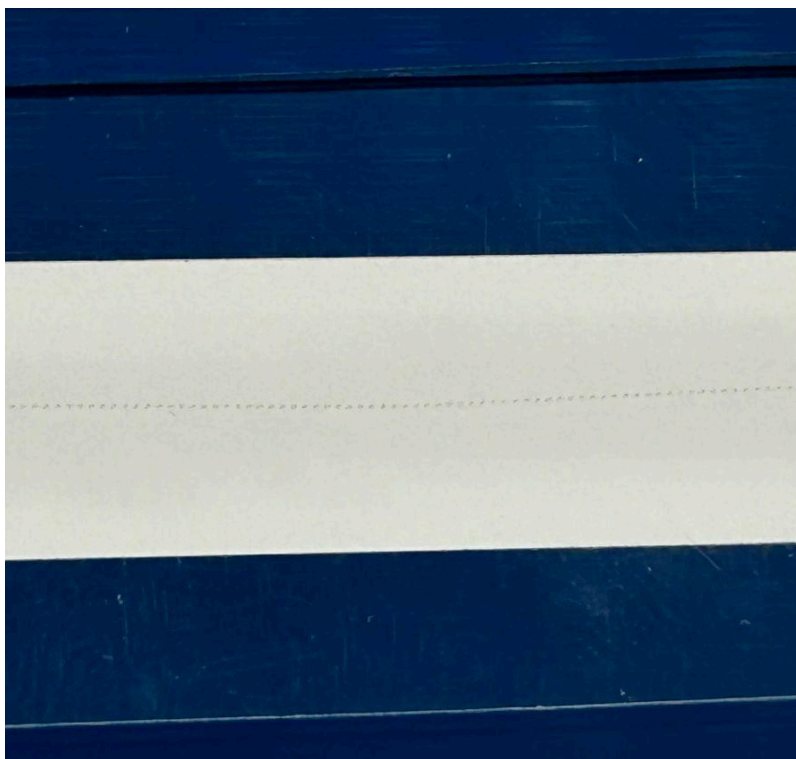
Figure 10. Shows a laser ablated mylar strip. The dots down the center are where the laser spot hit. The spots are around 0.2 mm in diameter.
