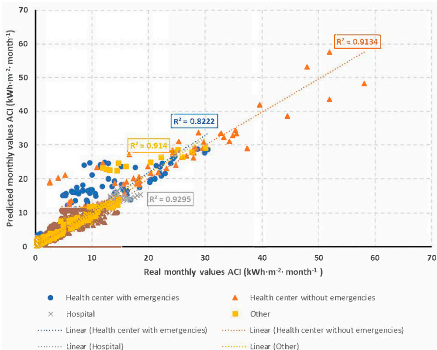
Figure 7. Correlation for each building type of the modeled values and the real data.
