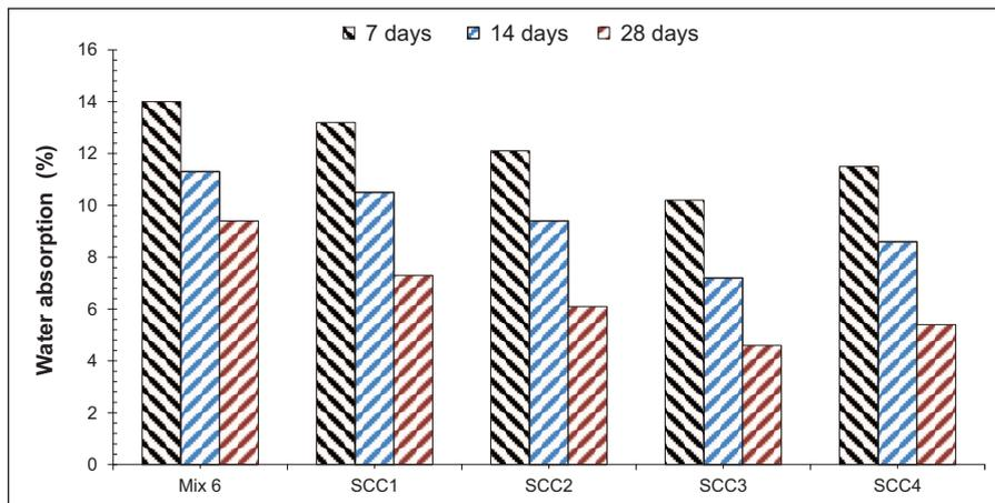
**Figure 7.** Water absorption of different samples at 7, 14, and 28 days.
