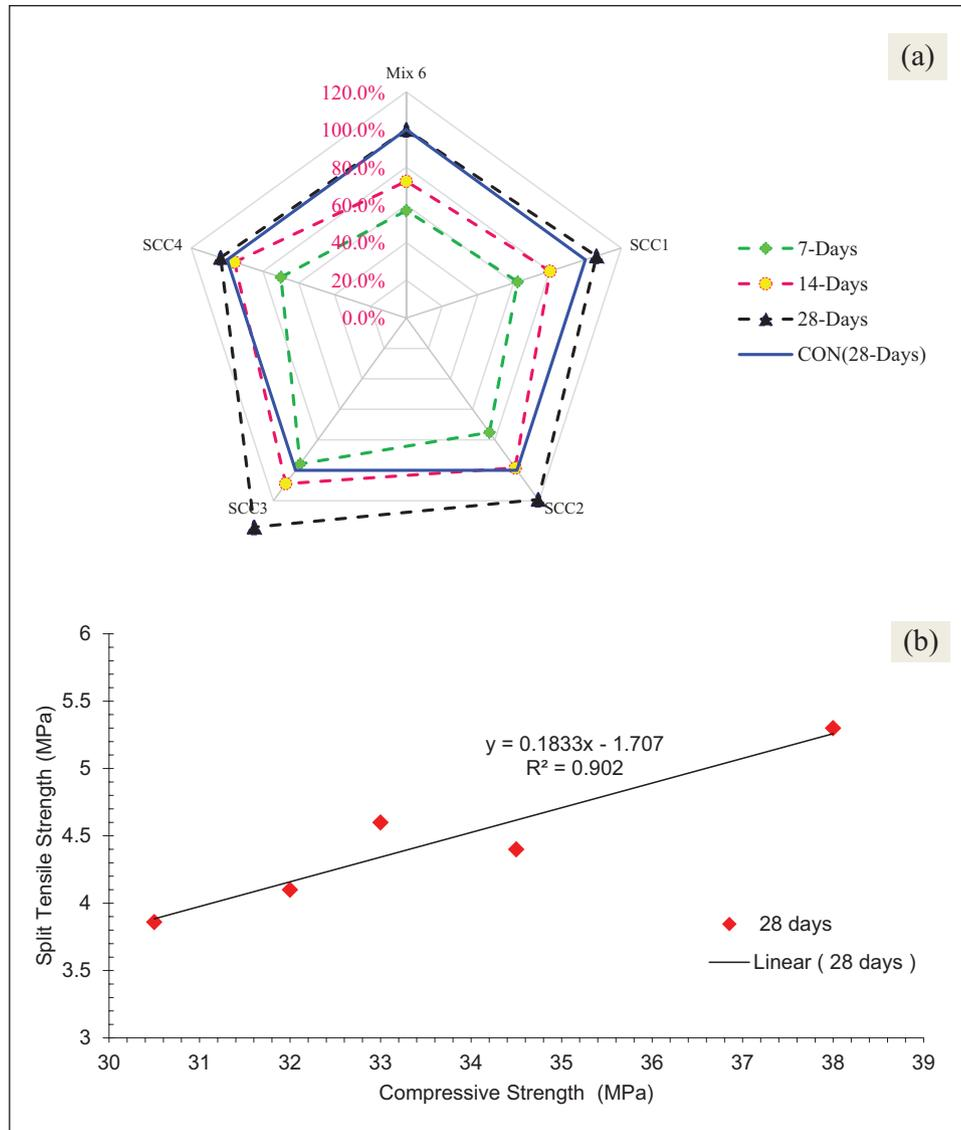
**Figure 6.** (a) Split tensile strength of each mix relative to 28 days strength of reference mix (Mix 6) and (b) co-relation between compressive strength and split tensile strength.
