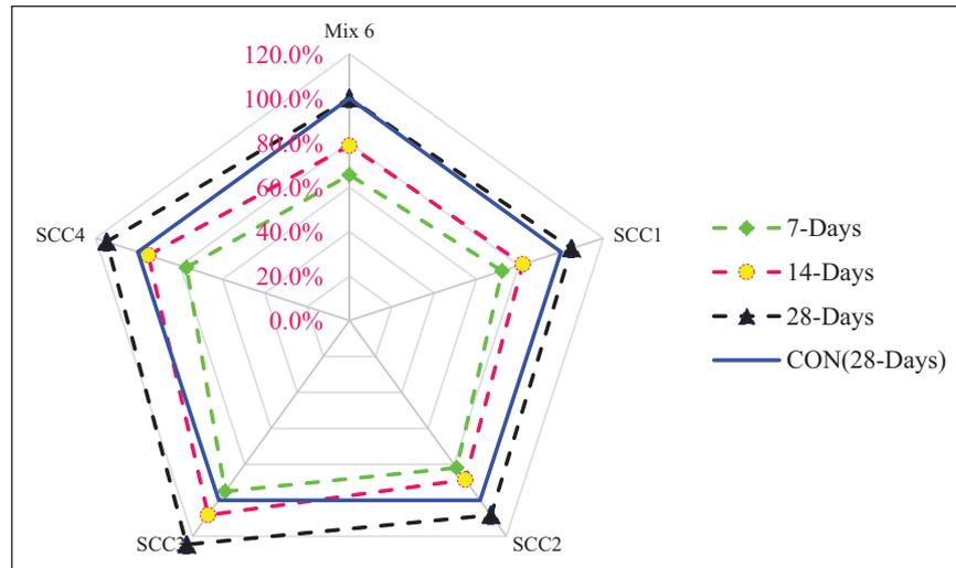
**Figure 4.** Compressive strength of each mix relative to 28 days strength of reference mix (Mix 6).
