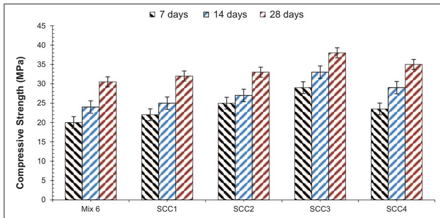
**Figure 3.** Compressive strength of different samples at 7, 14, and 28 days.
