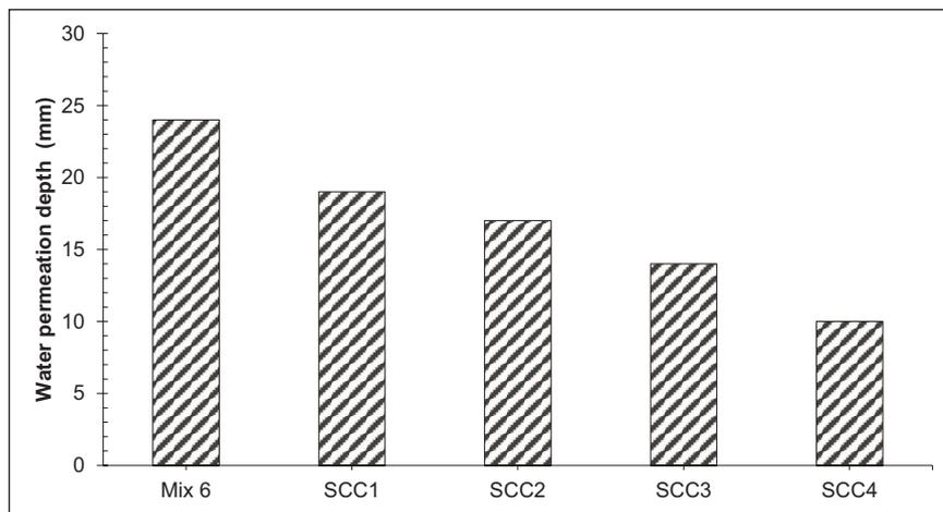
**Figure 9.** Permeability of the self-compacting concrete containing nylon fibers.
