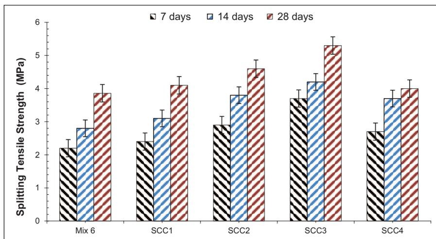
**Figure 5.** Splitting tensile strength of the samples at 7, 14, and 28 days.
