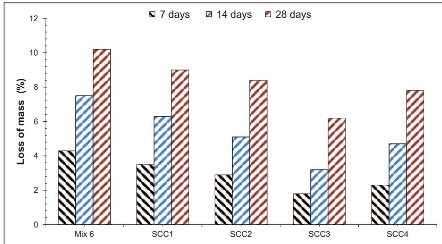
**Figure 8.** Percentage loss in concrete mass due to acid attack.
