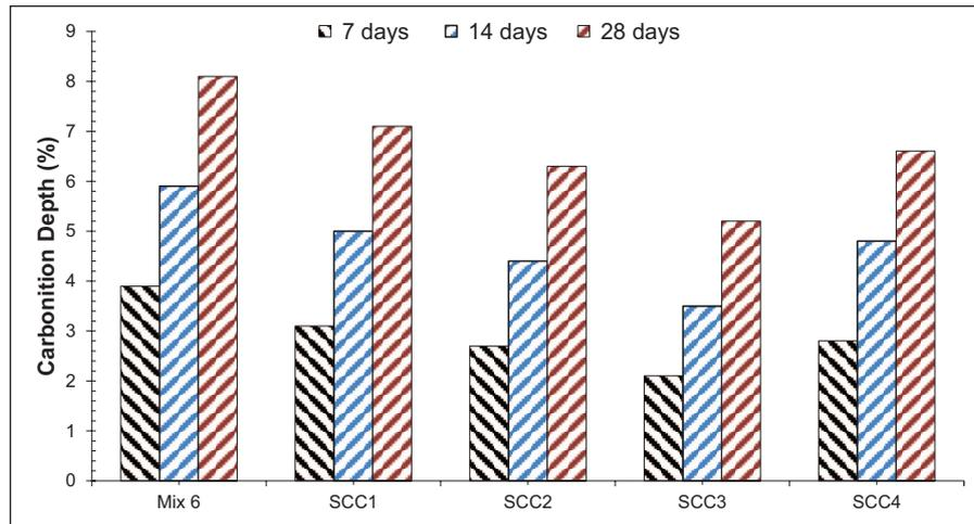
**Figure 10.** Carbonation resistance of the different samples.
