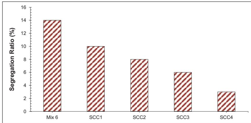
**Figure 2.** Segregation ratio of different mixes.
