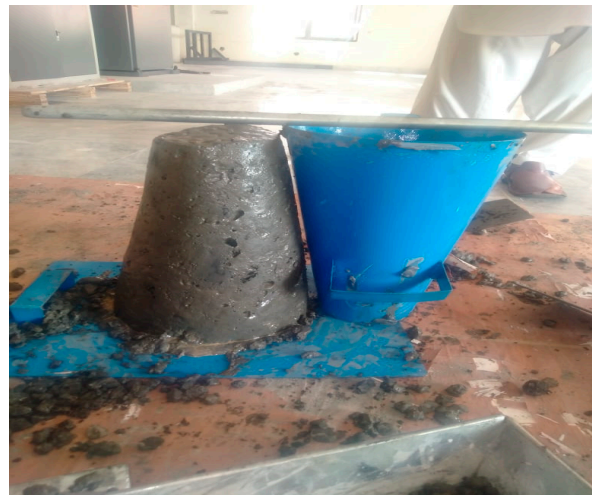
Figure 3. Slump test setup.
