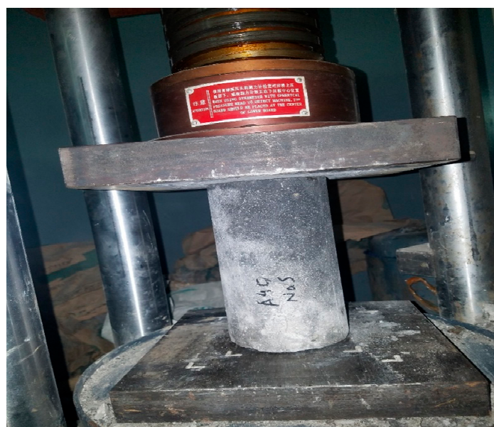
Figure 6. Compressive strength test setup.
