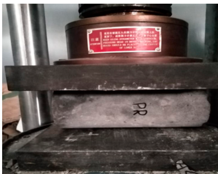
Figure 9. Split tensile strength test setup.
