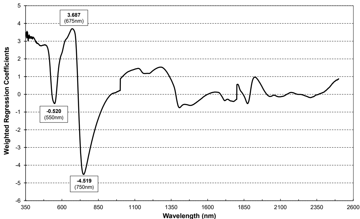
Figure 6. Weighted Regression Coefficients of PLS regression for estimation of infestation levels using reflectance values of dataset 1 (31 July) as prediction variables.
