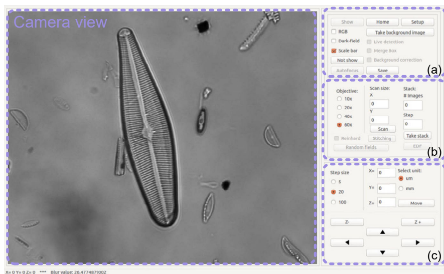
Figure 9. Main GUI window showing the camera view and the control panels: (a) configuration panel, (b) scanning and processing settings panel, and (c) motorized stage control panel.
