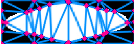
Fig. 10. Keypoints and Delaunay triangulation.
