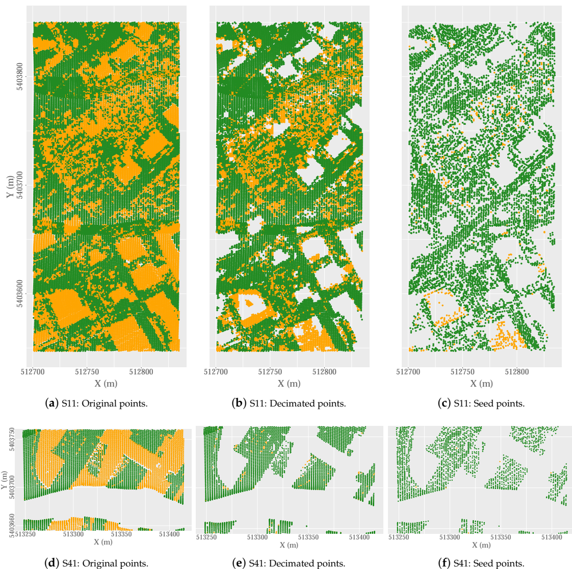
Figure 9. Qualitative results of the DecHPoints function (ground points in green and non-ground points in yellow). Examples: (a–c) are the results of Sample 11 and (d–f) the results of Sample 41.
