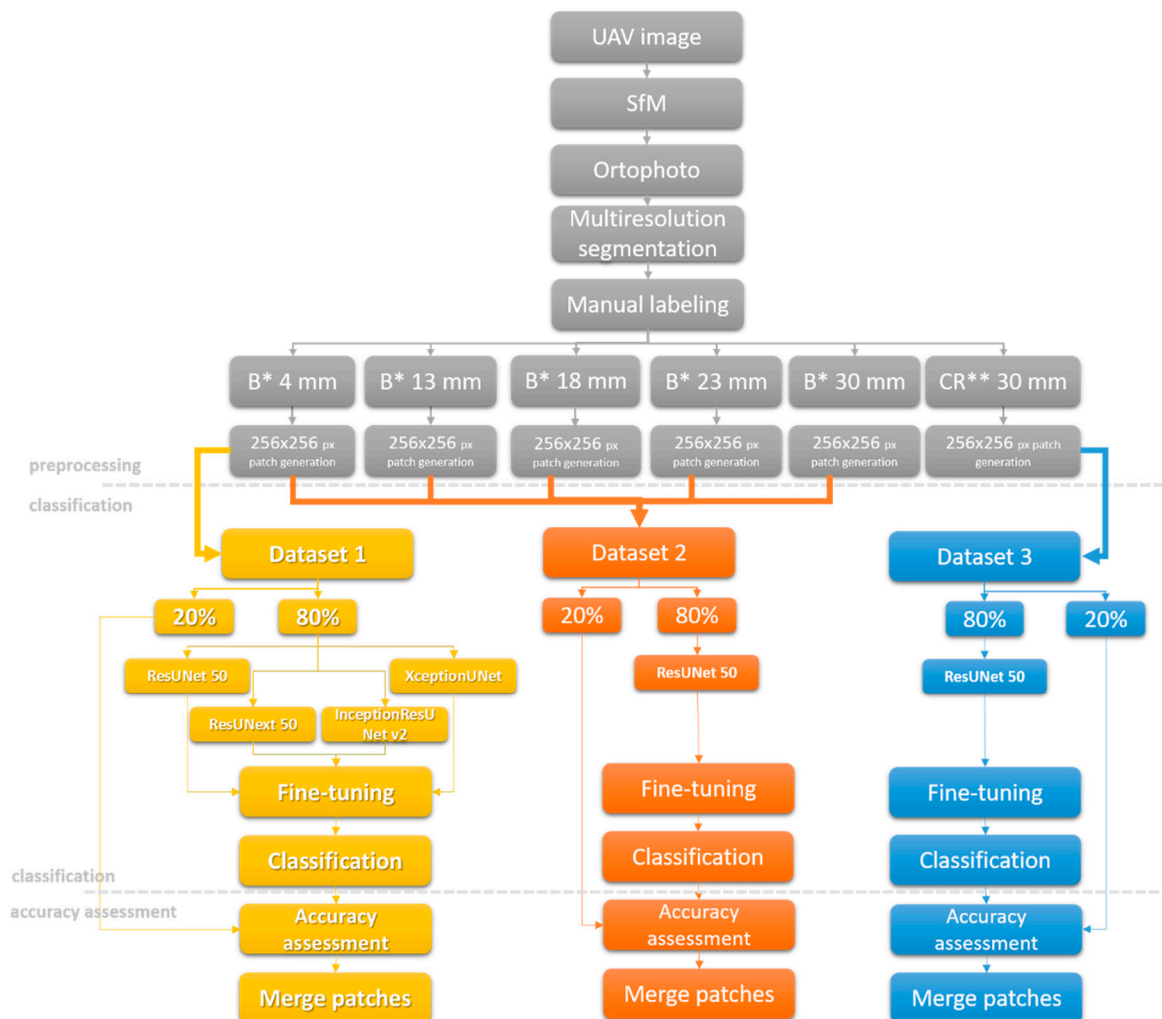
Figure 3. Workflow used in this study where “B*” and “CR**” correspond with the Balkana and Crna Rijeka dataset respectively. UAV = Unmanned Aerial Vehicles; SfM = Structure from Motion.
