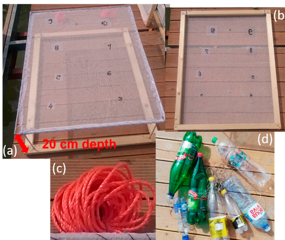
Figure 2. Targets used in the study area located in Lake Balkana (a) frame with metal construction for the underwater survey, (b) frame for the on the water surface survey, (c) nylon rope, (d) plastic bottles.
