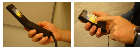
Fig. 3. Handset grips, one hand (OH) for H2 (left) and two hand (TH) for H1 (right).
