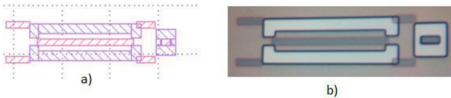
Figure 38 a) Photomask layout of laser ridge and ion implant mask b) Micrograph of processed device at the ion implant step.
