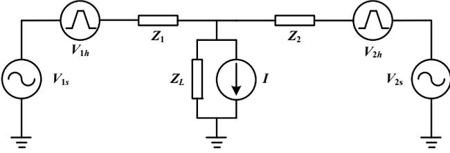
Fig. 5. Equivalent circuit of an islanded microgrid.
