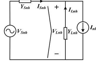
Fig. 7. Simplified equivalent circuit of the islanded microgrid.
