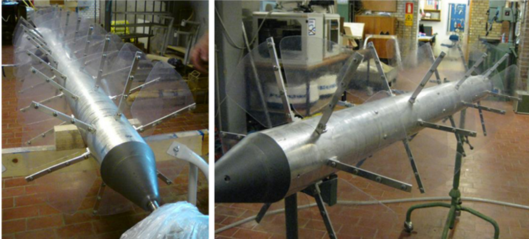
Figure 15. Investigation of number of fin's sets; seven (left) and four (right) with 0.75 mm thickness.
