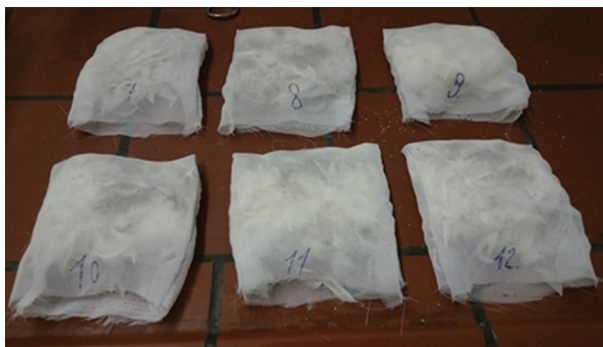
Figure 2. Composite pillows made from loose feathers and sepiolite in PET fabric.
