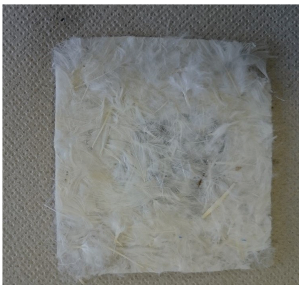
Figure 3. Composite sample (FS-sheet) prepared from feathers and sepiolite.
