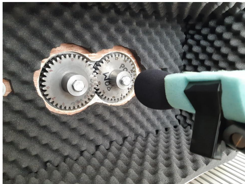
Figure 4. The tested gear pair on the testing device with the soundproof acoustic foam for acoustic soundproof insulation.
