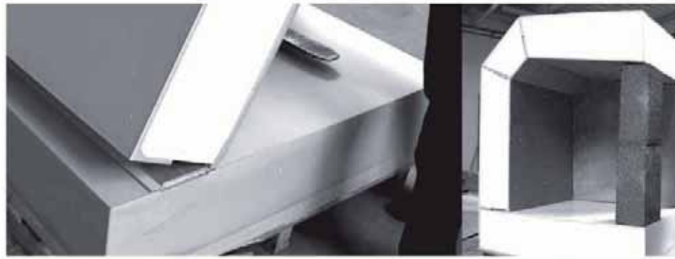
Figure 4: Prototype Envelope with 12 mm Face Sheets and 300 mm Insulation Core, thus a Highly Insulated but thin and Tight Envelope
