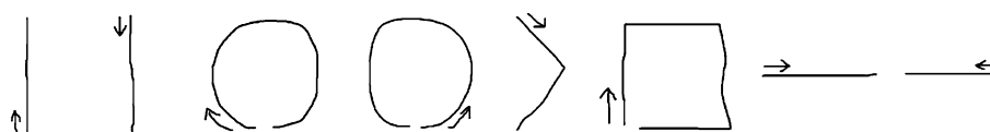
Fig. 4 VCR control gestures: From left to right gestures for play, stop, next, previous, increase, decrease, fast forward, fast rewind
