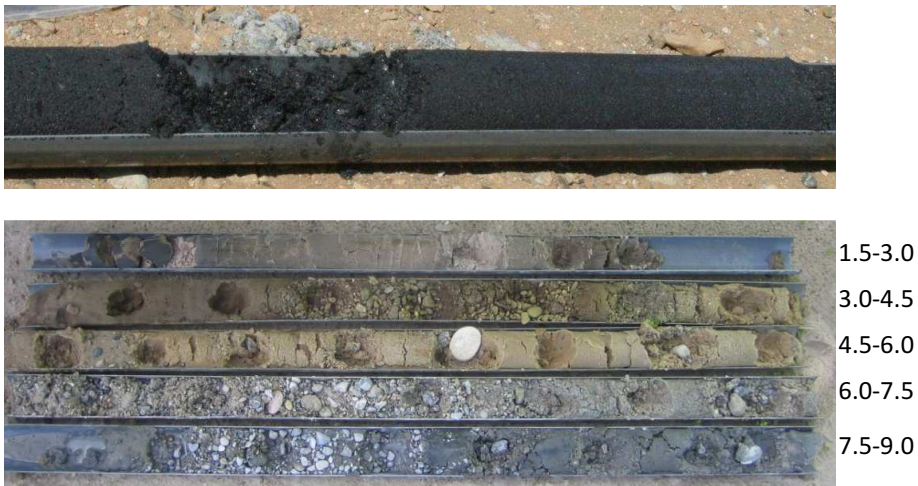
FIGURE 4-9: EXAMPELS OF INTACT SOIL CORES COLLECTED FROM THE TREATMENT AREA BEFORE MFR INJECTIONS (UPPER) AND AFTER TWO INJECTION EVENTS (LOWER, WITH DEPTH INTERVALS IN M BGS). THE CORES ALSO ILLUSTRATES THE LAYERED GEOLOGY.
