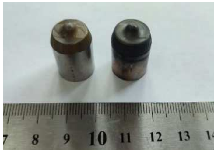
Figure 2. FSW tool before (left) and after (right) welding.
