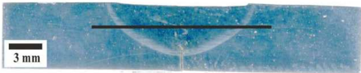
Figure 3. Cross section of the FSW joint sample.
