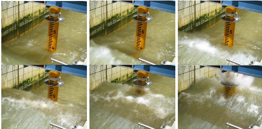
Fig. 1: Large scale testing of loads on wind turbine access platforms.
