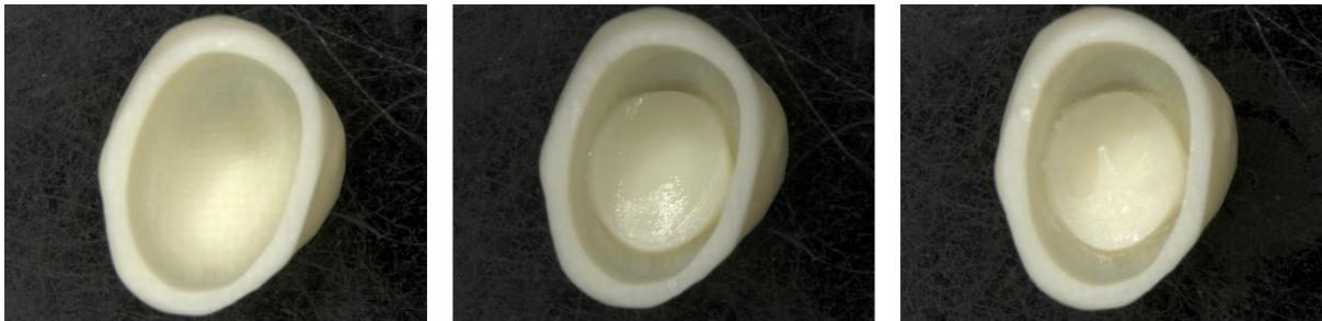
Fig. 10: Microscopic images of the secondary crown surface (12×). Left image: without an OS before the insertion/removal tests. Center image: with an OS before the insertion/removal tests. Right image: with an OS after the insertion/removal tests.
