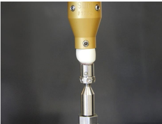
Fig. 2: All samples were tested using a universal testing device with a fitting force of 100 N.
