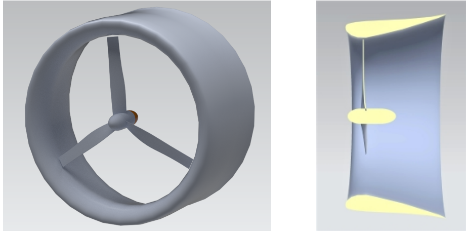
Figure 5: 3D CAD and section cut view of the DonQi DAWT.
