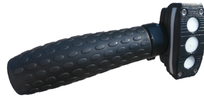
Figure 4: The final version of Tribike with three action buttons. The device uses the same button patterns as standard mobile phone in-line remotes.
