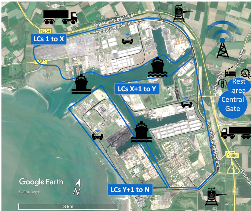
Figure 8. SLN at the Port of Vlissingen East (PoV) with a Central Gate, i.e. a decoupling point (DP) incorporating a rest area and trailer services (Brunetti, Mes, and Van Heuveln 2020).
